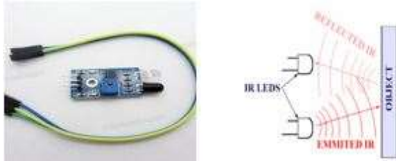
Fig.5. IR obstacle avoidance sensor & object detection using IR sensor.
